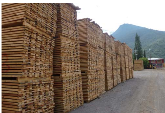
Open air drying of wood, Mexico. Photo: Industria Forestal Pueblos Mancomunados
